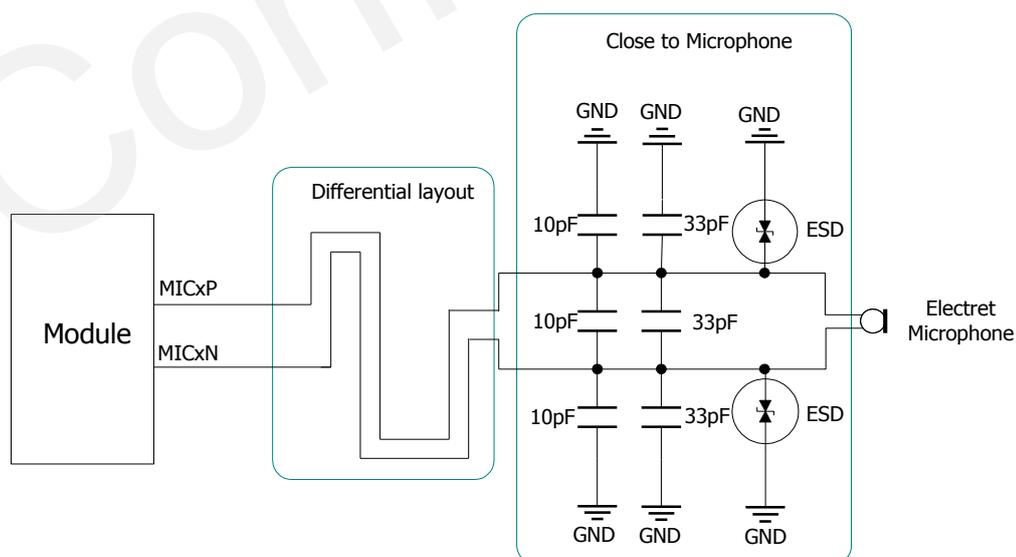
**Figure 31: Microphone interface design of AIN1&AIN2**
