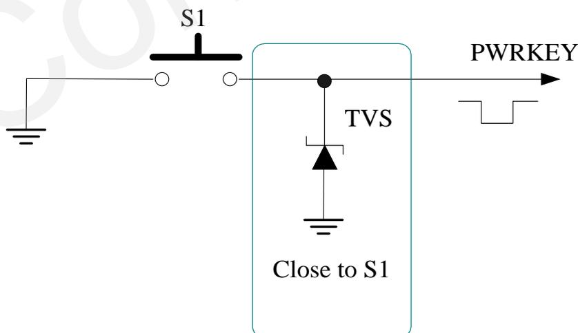
Figure 7: Turn on the module using keystroke
