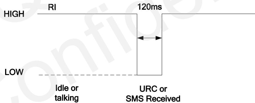
Figure 44: RI behaviours of URC or SMS received
