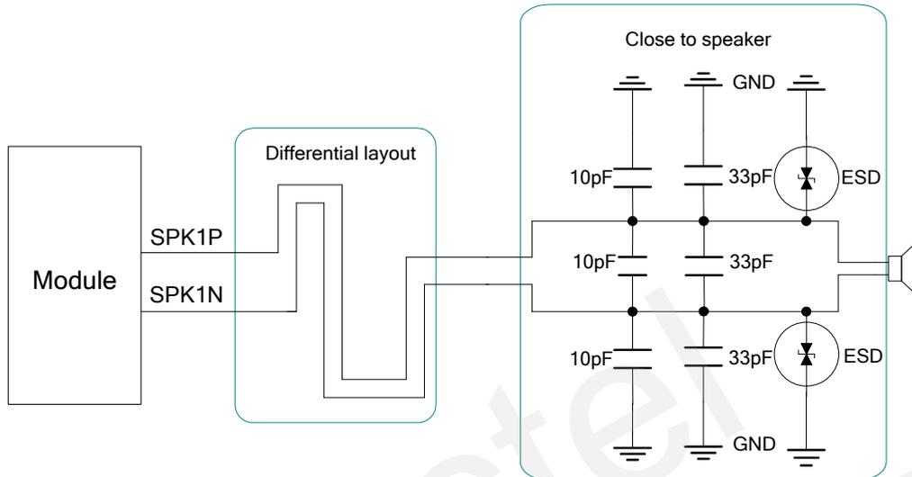
**Figure 32: Receiver interface reference design of AOUT1**
