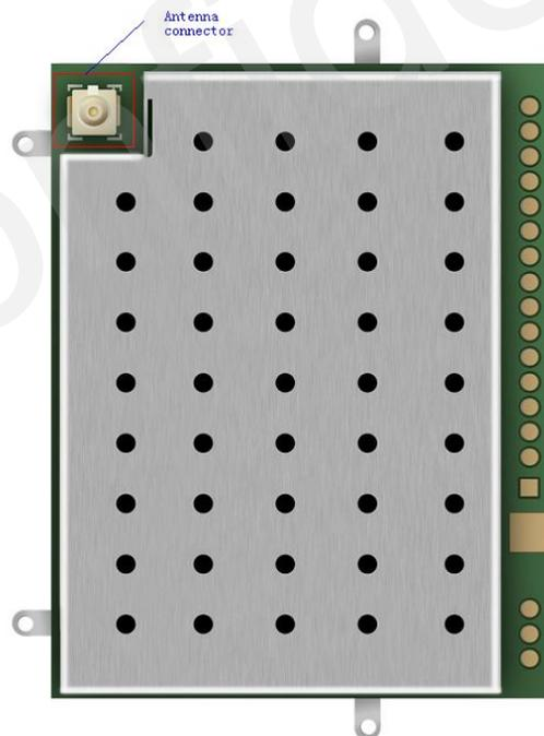
Figure 47: Antenna connector
