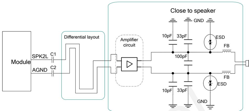
**Figure 35: Speaker interface with amplifier design of AOUT2**
