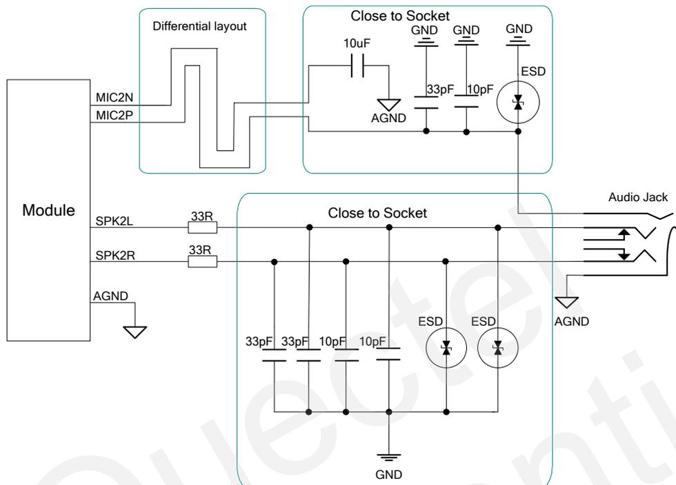
**Figure 34: Earphone interface design**
