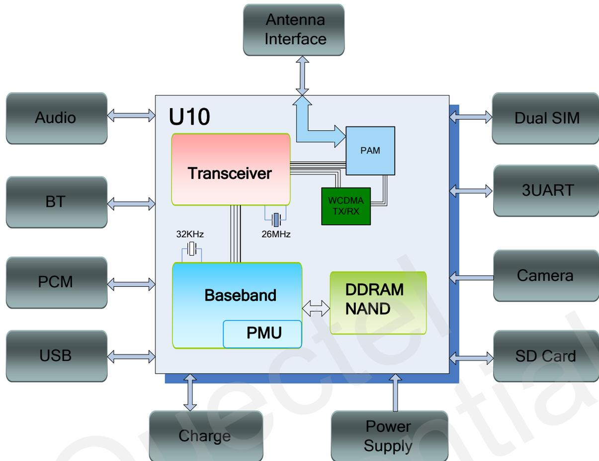
Figure 1: Module functional diagram
