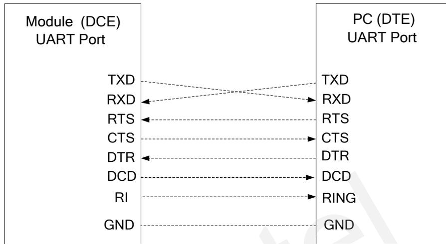
**Figure 18: Connection of full function UART port**
