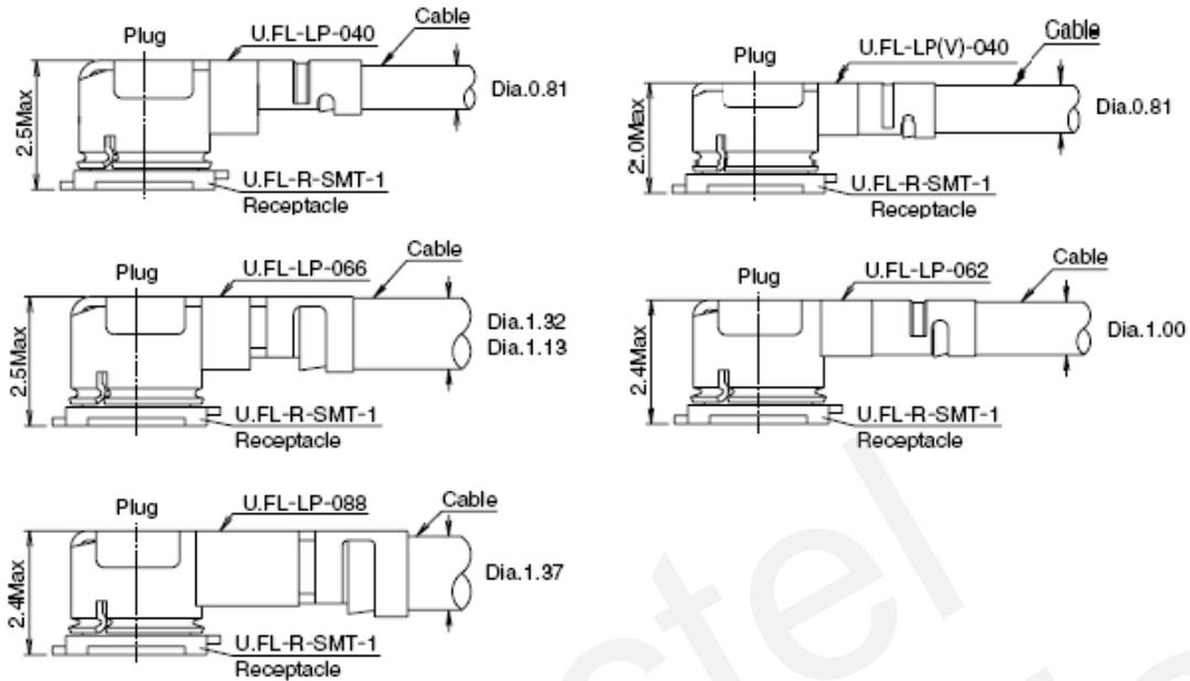
**Figure 50: Space factor of mated connector (Unit: mm)**
