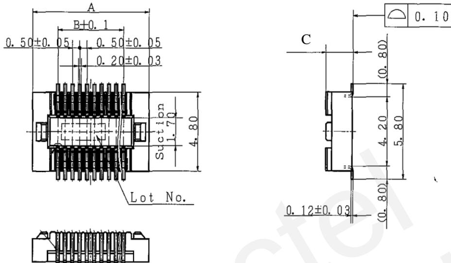
Figure 55: Sketch map of 100 pin board to board socket (Unit: mm)
