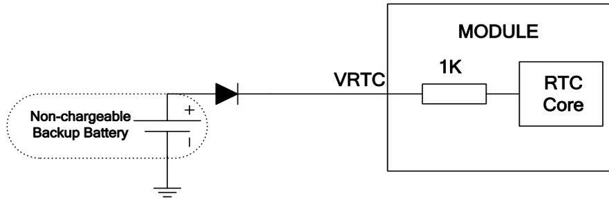
Figure 14: RTC supply from non-chargeable battery
