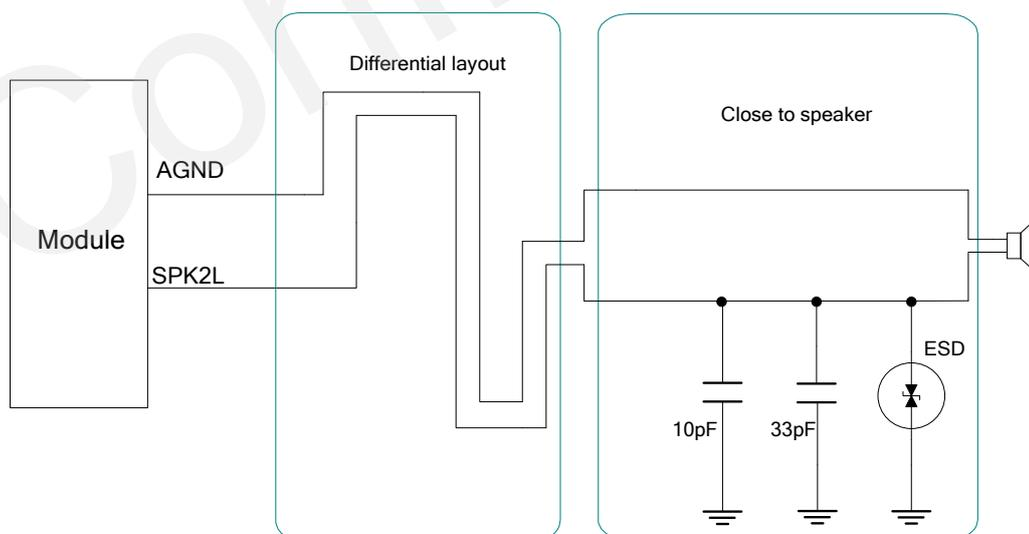
**Figure 33: Single side design of AOUT2 with SPK2L**
