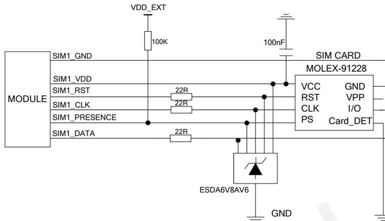
**Figure 27: Reference circuit of the 8-pin SIM card**
