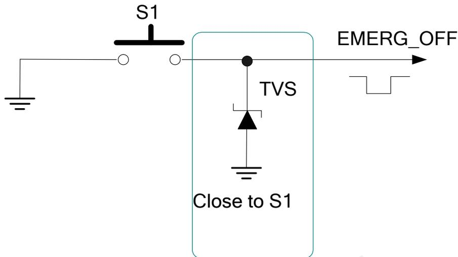
Figure 11: Reference circuit for EMERG\_OFF by using button
