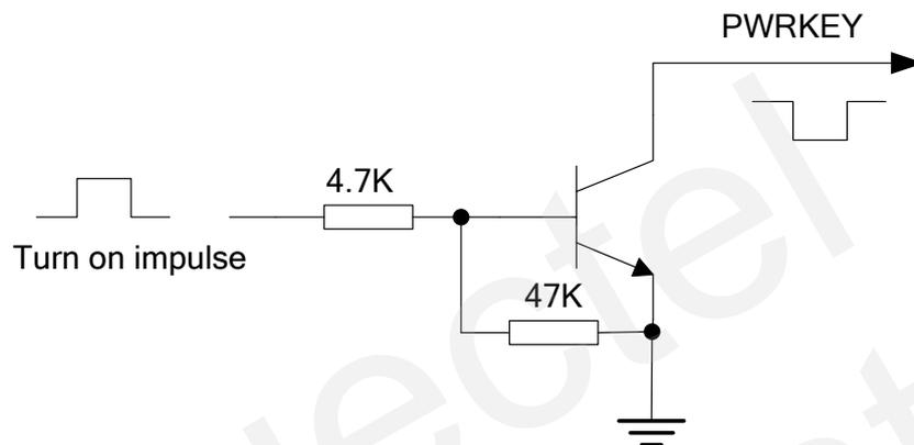
Figure 6: Turn on the module using driving circuit
