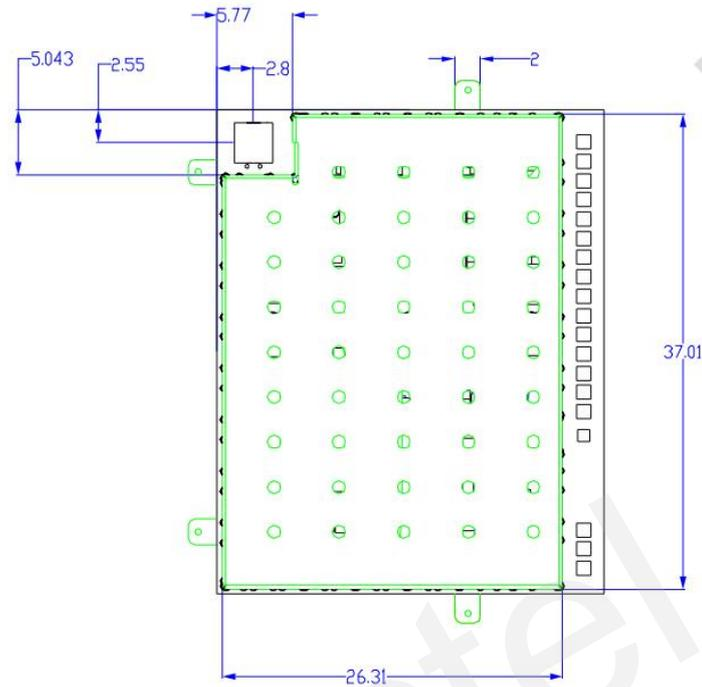
Figure 53: U10 BOT dimension (Unit: mm)
