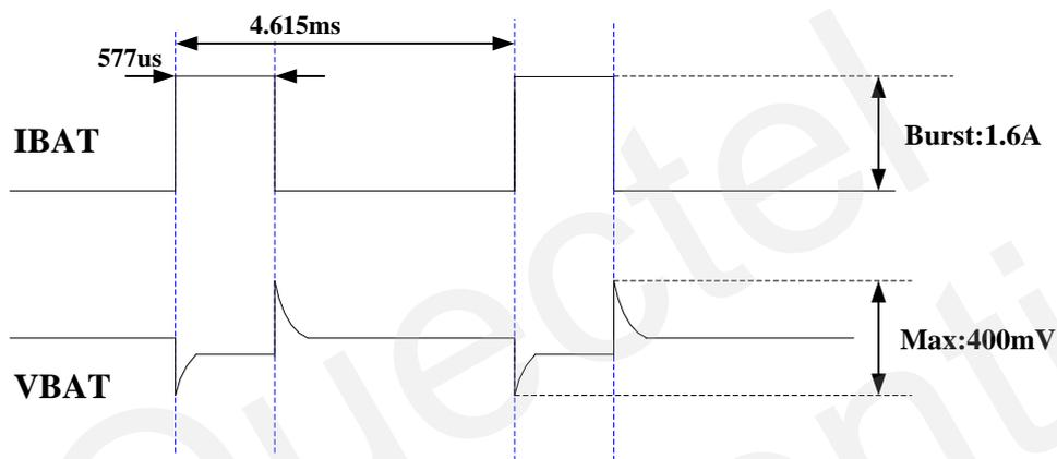
Figure 2: Ripple in supply voltage during transmitting burst
