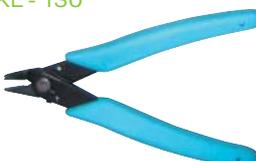
Precise electronic pliers with insulated handles, for wires up to 0,8mm diameter. With a spring for collecting ends of wires that have been cut off, cutter angled at 20°. Length: 130mm.
