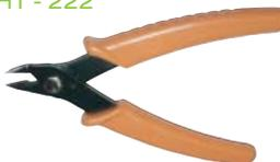
Precise electronic pliers, cutter angled at 22,5°, made of finest tool steel, black burnished surface, spring-loaded, Length: 130mm, for copper wire up to 0,79mm<sup>2</sup> (AWG18).
