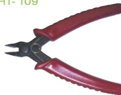
Flat profile electronic pliers. High-leverage design provides greater cutting and gripping power, cutter angled at 22,5°, made of finest tool steel, induction hardened, black burnished surface. Spring-loaded, Length: 130mm, for copper wire up to 0,519mm<sup>2</sup>.
