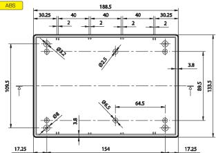
Part No. Description, dimensions A x B x C (LxWxH) TK22.9 TEKMAR ABS enclosure 188,5x133,5x55,5mm black
