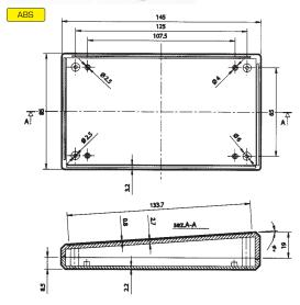
Description, dimensions A x B x C (LxWxH) Part No. 450S.9 TENCLOS ABS enclosure for desktop 145x85x27,5mm black
