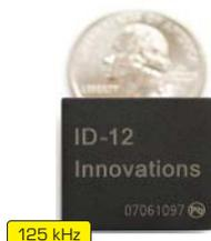
The ID2, ID12 and ID20 are similar to the obsolete ID0, ID10 and ID15 MK(ii) series devices, but they have extra pins that allow Magnetic Emulation output to be included in the functionality. The ID-12 and ID-20 come with internal antennas, and have read ranges of 12+ cm and 16+ cm, respectively. With an external antenna, the ID-2 can deliver read ranges of up to 25 cm. All three readers support ASCII, Wiegand26 and Magnetic ABA Track2 data formats.
